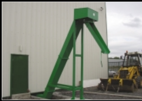
Outside Discharge Conveyor with swivelling chute for maximum Swarf dispersal.
